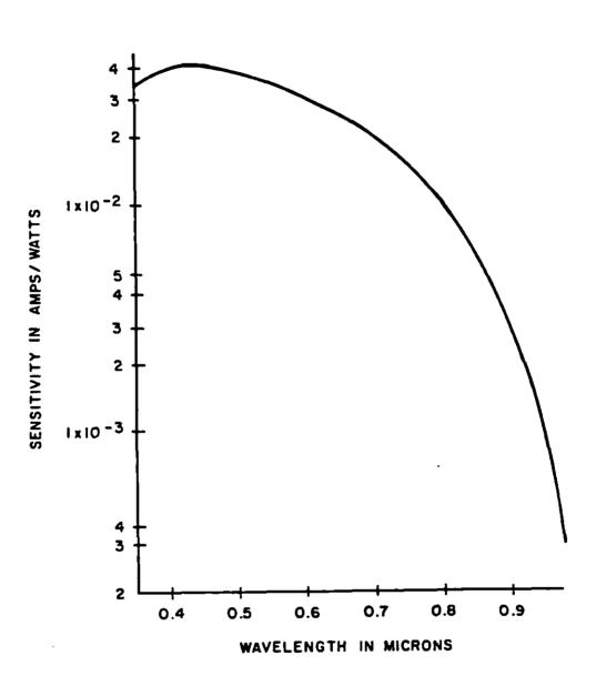
FIG. 1. S-20 EXTENDED RED RESPONSE CURVE
