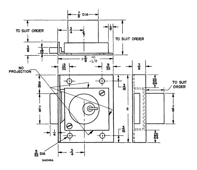
Figure 2 - Type B locks for metal and wood drawers.
