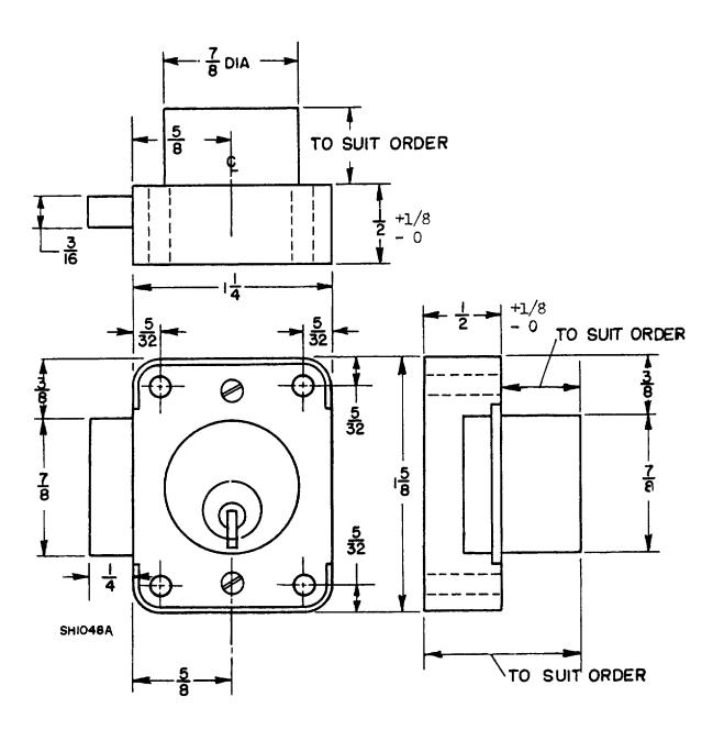
Figure 1 - Type A locks for metal and wood doors.
