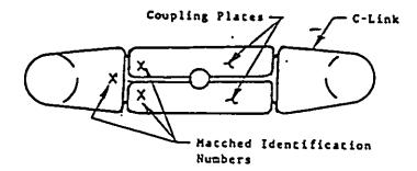
FIGURE 1. Location of C-link and coupling plates identification numbers.
