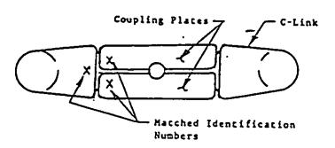
FIGURE 1. Location of C-link and coupling plates identification numbers.
