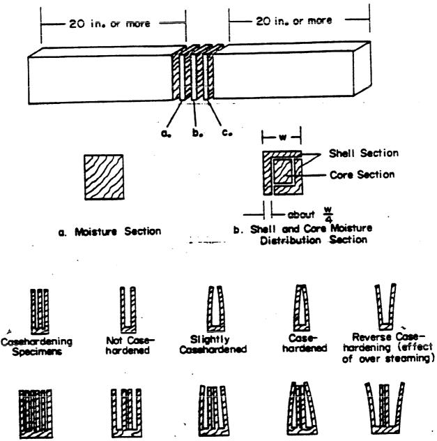
c. Casehardening - Material that is less than 1-1/2 inches thick is cut into three prongs, and the middle prong removed, material that is 1-1/2 inches thick or thicker is cut into six prongs, and the second and fifth prongs removed.
