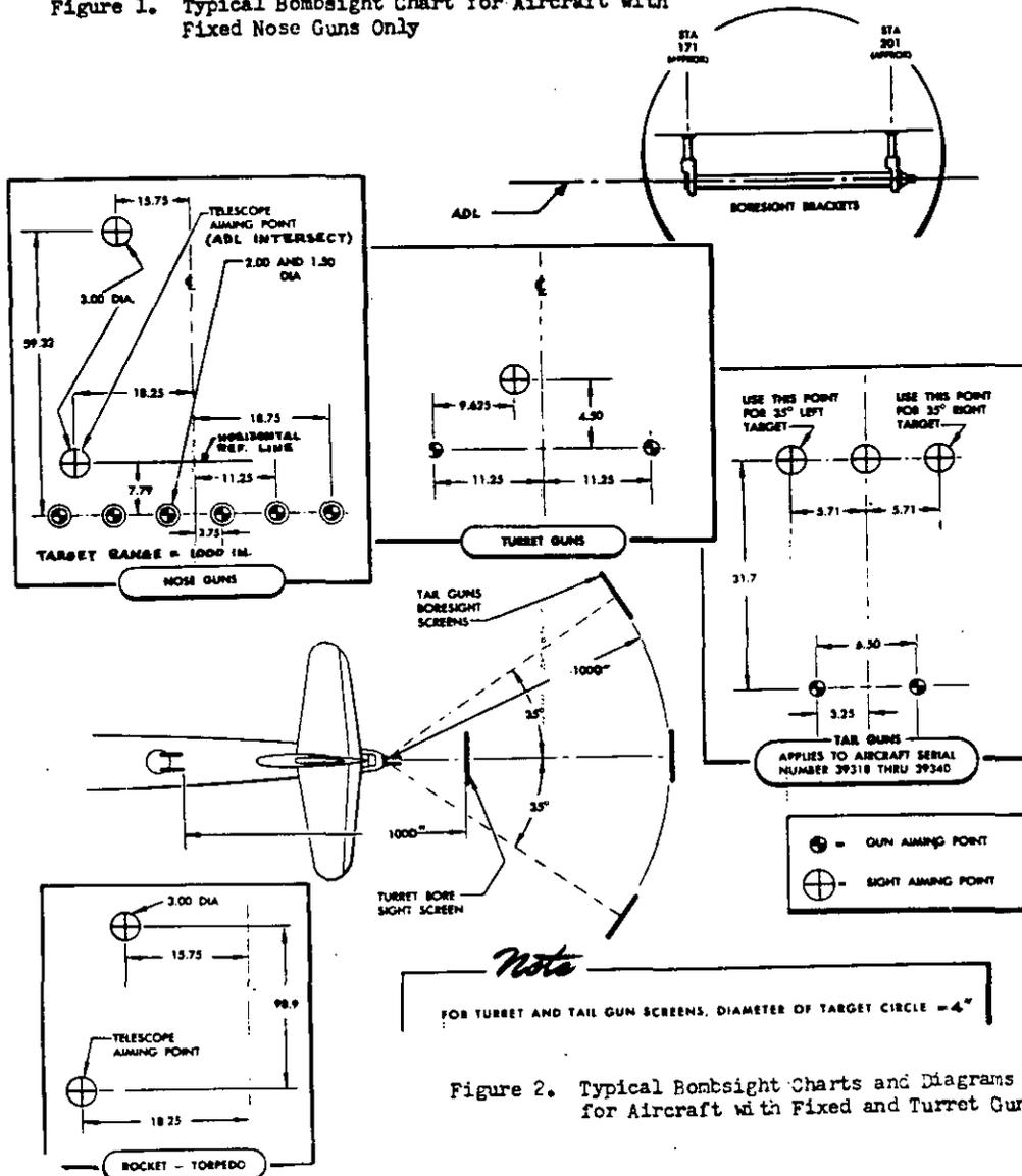
Figure 2. Typical Bombsight Charts and Diagrams for Aircraft with Fixed and Turret Guns
