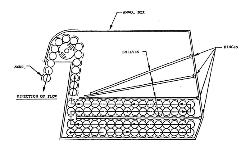
FIGURE 1. Typical layer-type ammunition box.
