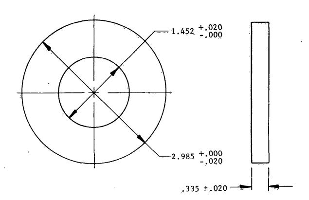
FIGURE 2. TYPE III COMPOUND (WAFER) (FOR MK 273 MOD 1 IGNITER ONLY)
