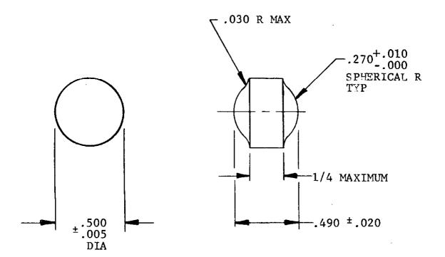
FIGURE 1. TYPE II, PELLET CONFIGURATION.
