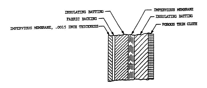
$\frac{1}{2}$  Optional construction is cloth backing supported in a heat sealable plastic (See 3.1.3.2).
