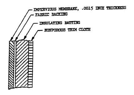
1/ Optional construction is cloth backing supported in a heat sealable plastic (See 3.1.3.2).
