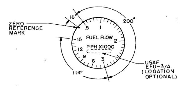
NOTE: 14,000 PPH GRADUATION TO BE MAINTAINED AT HORIZONTAL CENTERLINE
