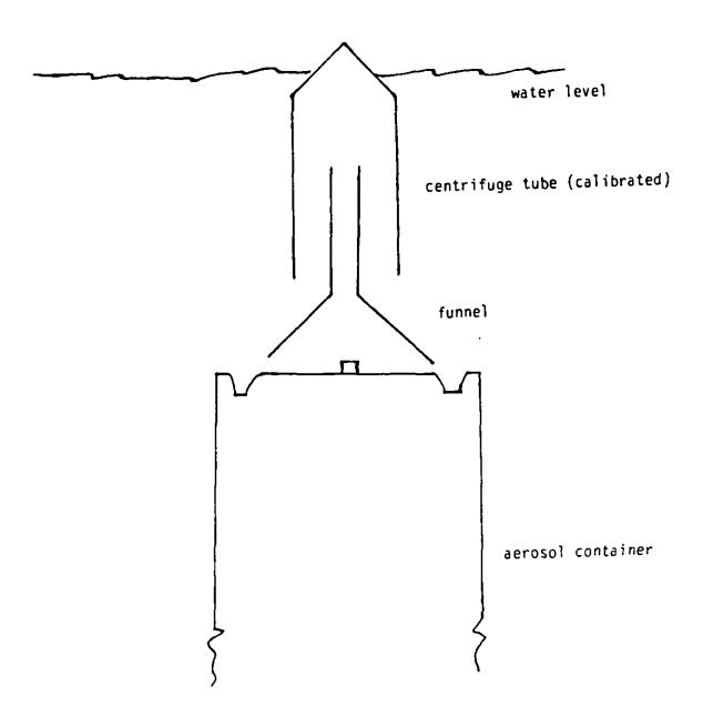
FIGURE 3. Apparatus for aerosol container volumetric leakage.
