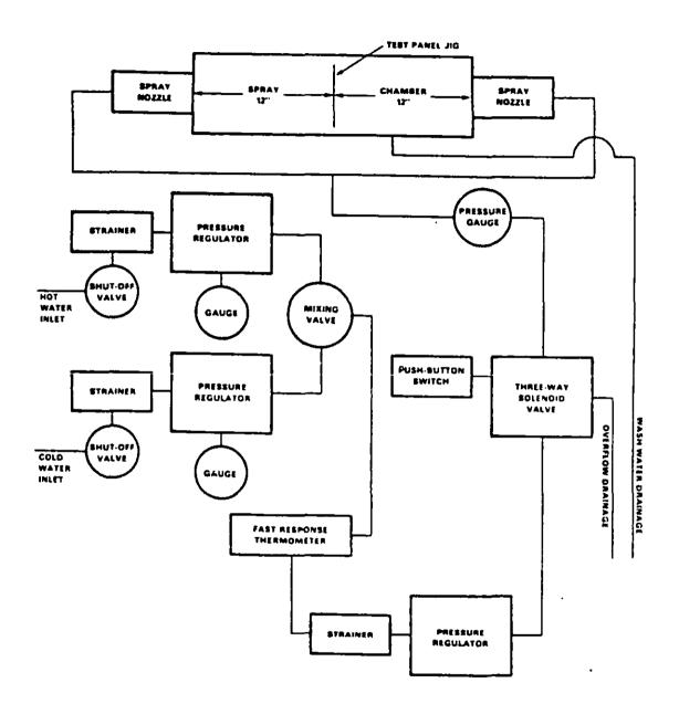
FIGURE 2. Penetrant removability test apparatus.
