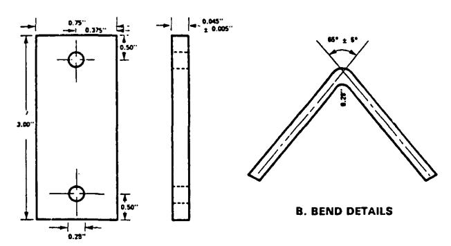
A. DIMENSION DETAILS (± 0.01" TOLERANCE EXCEPT THICKNESS)
