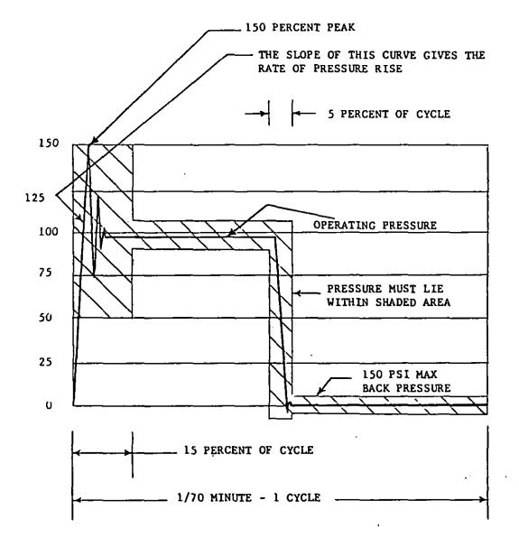
FIGURE 2. DYNAMIC PRESSURE IMPULSES
