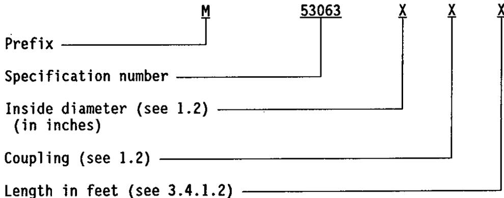
Example of part number: M53063-3-5-3 for a 3-inch diameter, 5 foot long hose assembly with quick disconnect, cam-locking type couplings, hole shank; female one end, and male other end, in accordance with this specification.
