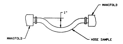
FIGURE 1. Horizontal steam rack.
