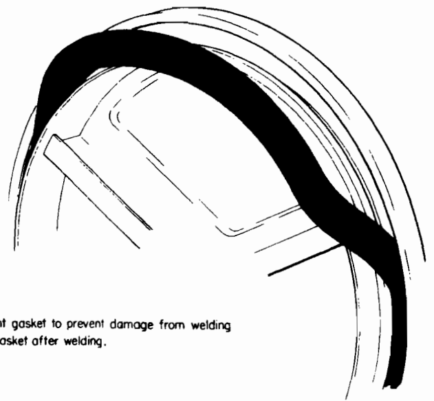
FIGURE 2. Installation procedures for left-hand or right-hand hinged armored doors swinging out to open, style 2.
