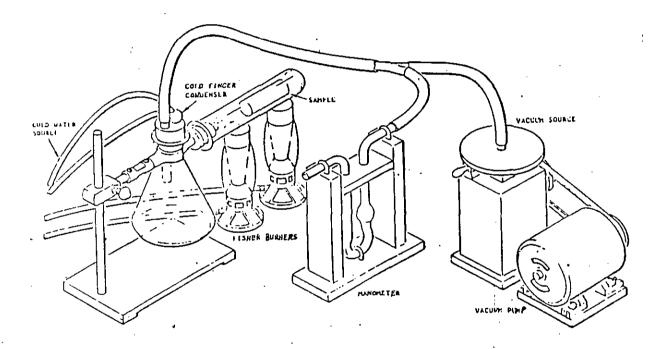
FIGURE 2. Resin content apparatus setup.
