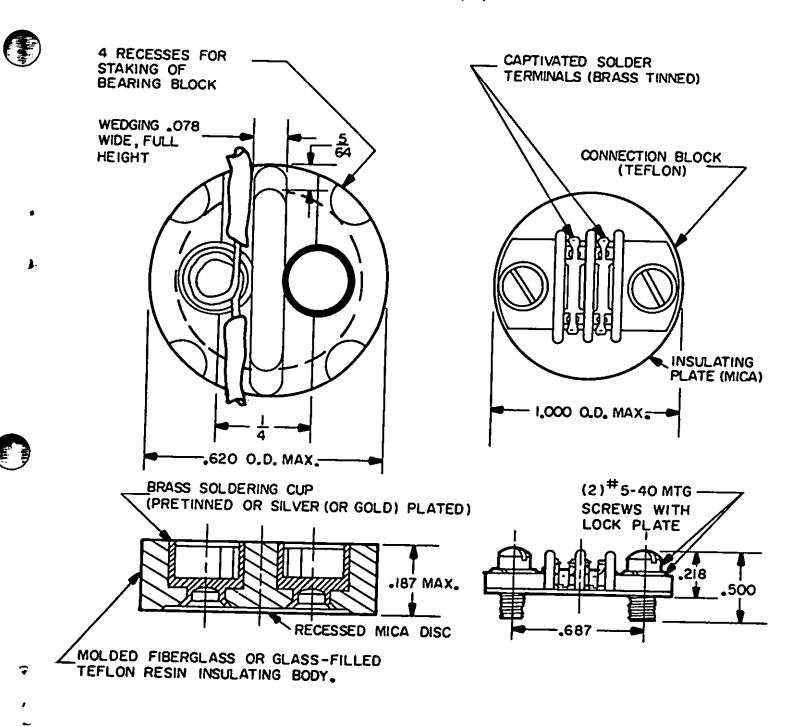
NOTE: A two-wire system is depicted; however, either a two- or three-wire system is acceptable.
