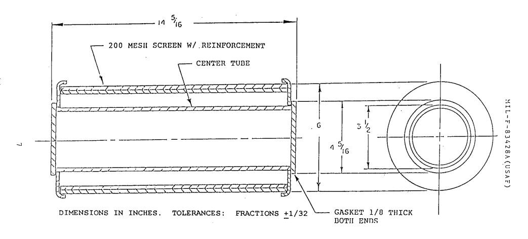
FIGURE 1. Filter element.
