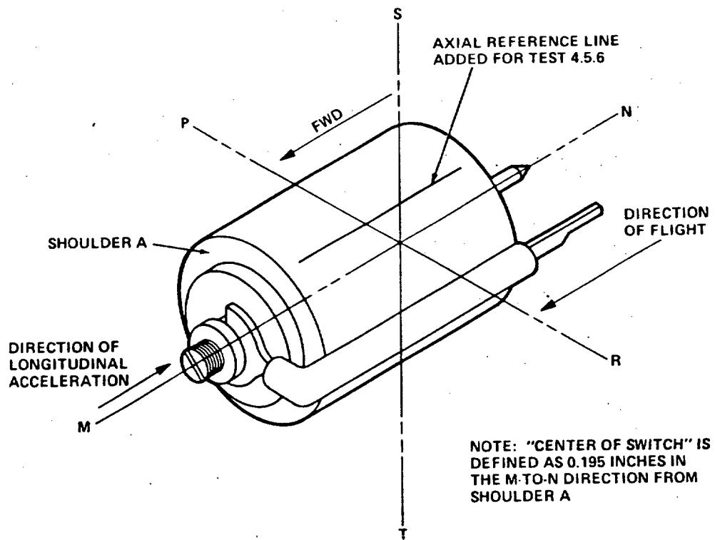
FIGURE 1. Impact switch assembly (9297012)
