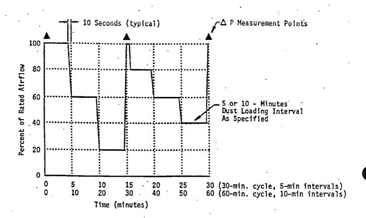
FIGURE 1. Variable airflow cycle.
