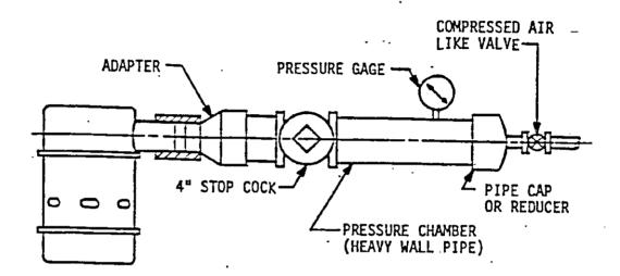
FIGURE 3. Backfire test setup.
