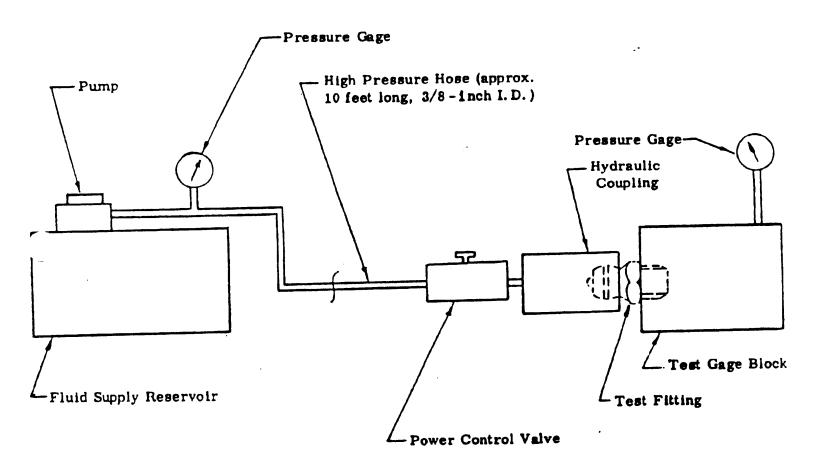
FIGURE 2. Leakage test setup.
