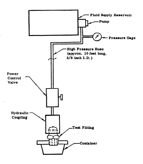
FIGURE 3. Blowout test setup.
