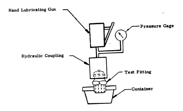
FIGURE 1. Extreme angular position and opening pressure test setup.
