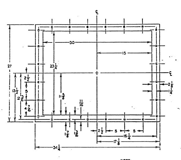
NOTE: STANDARD TOLERANCE OF ALL CRITICAL BOLT HOLE LOCATION DIMENSIONS SHALL BE ± 0.010.
