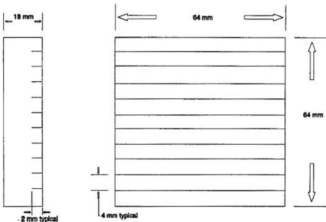
FIGURE 1. Abrader dimensions.
