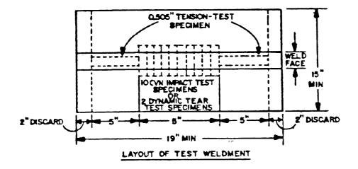
Base plate size shall be increased to provide additional Charpy (or dynamic tear) test specimens as required.
