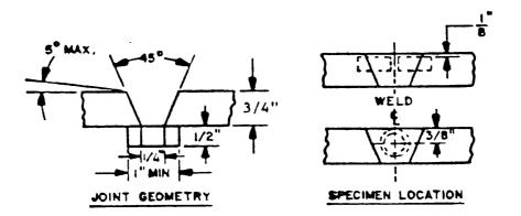
Maximum weld reinforcement shall not exceed 1/8 inch.
