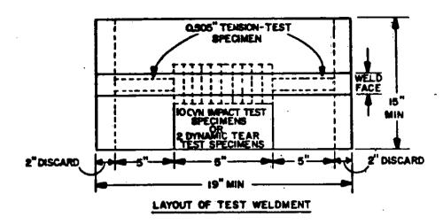
Base plate size shall be increased to provide additional Charpy (or dynamic tear) test specimens as required.
