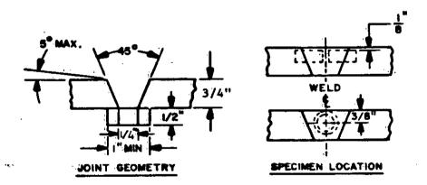
Maximum weld reinforcement shall not exceed 1/8 inch.
