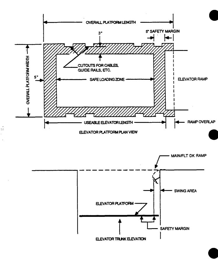
FIGURE 5. <u>Weapons-elevator safety margin</u>.
