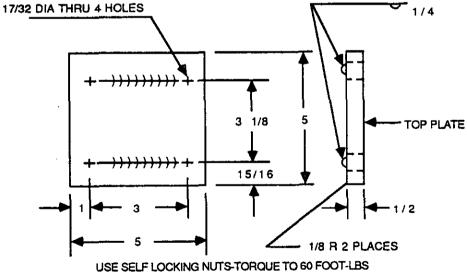
FIGURE 1. Wire rope clamp for hoist drum.
