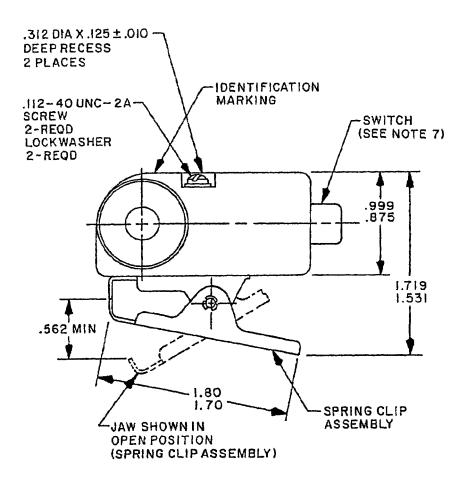
FIGURE 1. Dimensions and configurations (M9177/5-1).
