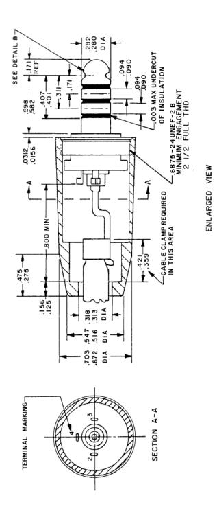
FIGURE 1. Dimensions and configutrations. - Continued.
