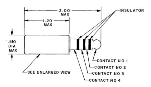
FIGURE 1. <u>Dimensions and configurations</u>.
