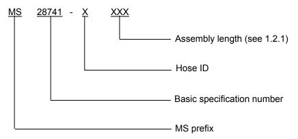
1.2.1 <u>Hose assembly length</u>. Length of hose assembly in inches. (Always use 3 digits. Use leading zeros as required.)
