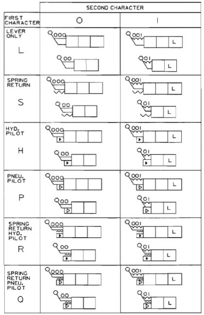
SYMBOLS 'I' AND 'L' INDICATES THE POSITION THAT THE VALVE SPOOL IS LATCHED OR DETENTED.
