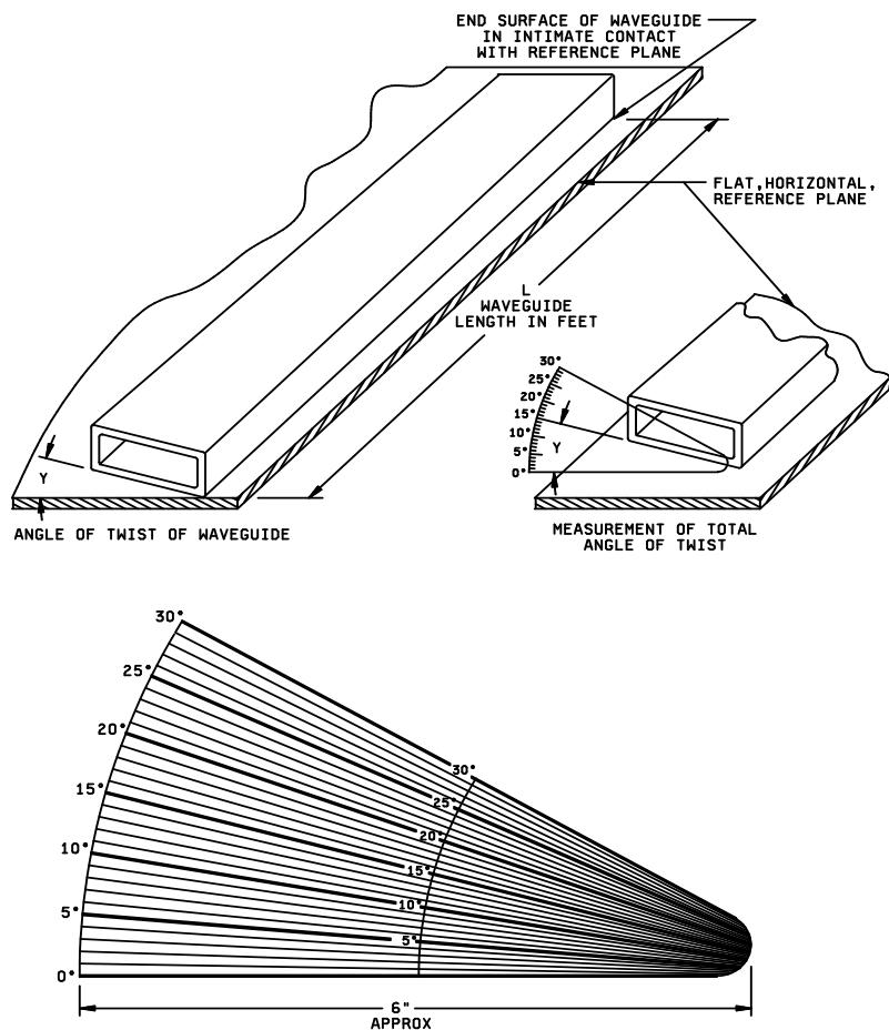
FIGURE 1. Method of determining twist.
