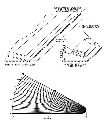
FIGURE 1. Method of determining twist.
