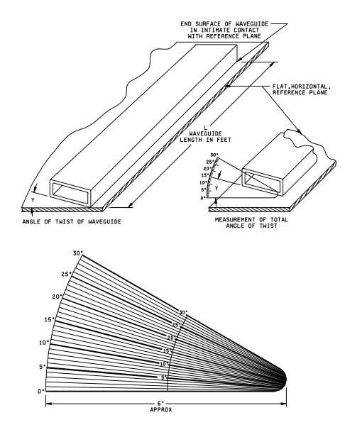
FIGURE 1. Method of determining twist.
