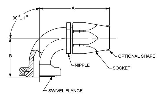
FIGURE 1. Fitting, swivel flange, 90 degrees.
