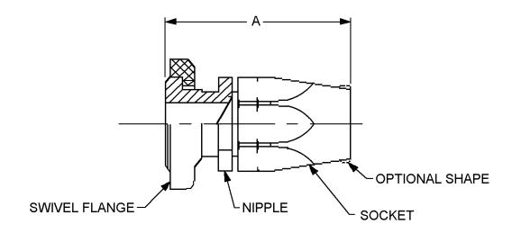
FIGURE 1. Fitting, swivel flange straight.
