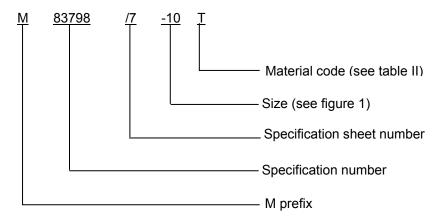
M83798/7-10L-T indicates: Straight swivel flange, 7/8 inch, titanium annealed.
