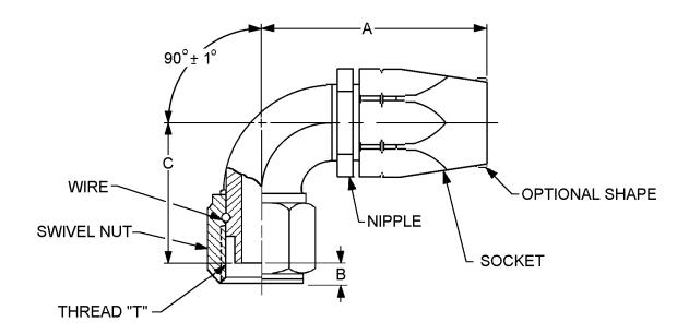
FIGURE 1. Fitting, flareless, swivel nut, 90 degrees.
