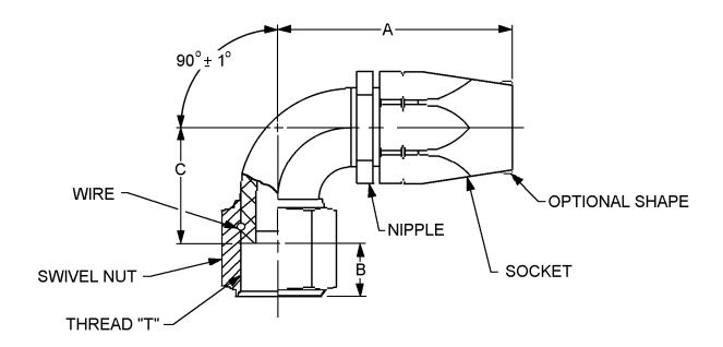
FIGURE 1. Fitting, flareless, swivel nut, 90 degrees.
