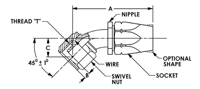
FIGURE 1. Fitting, flareless, swivel nut, 45 degrees.
