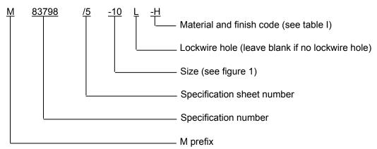
M83798/5-10L-H indicates: 7/8" Fitting, flareless, swivel nut, 45 degrees, with lockwire hole, with zinc phosphate finish on nipple and nut.
