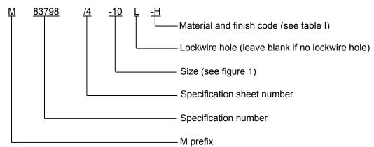
M83798/4-10L-H indicates: 7/8" fitting, flareless, swivel nut, straight, with lockwire hole, with zinc phosphate finish on nipple and nut.
