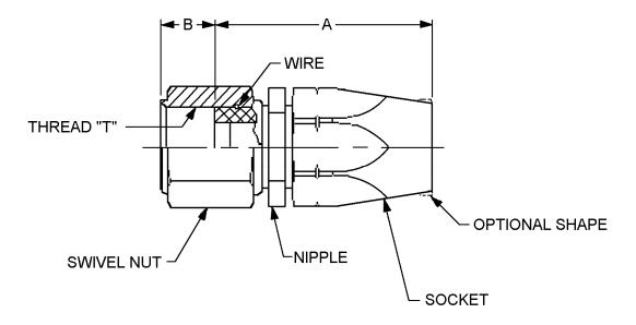
FIGURE 1. Fitting, flareless, swivel nut, straight.
