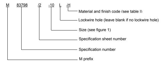
M83798/2-10L-H indicates: 7/8 inch fitting, flared, swivel nut, 45 degrees, with lockwire hole, and zinc phosphate finish on nipple and nut.
