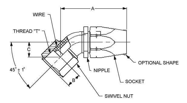
FIGURE 1. Fitting, flared, swivel nut, 45 degrees.
