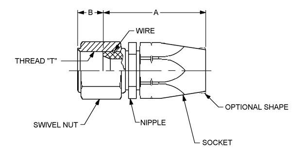
FIGURE 1. Fitting, flared, swivel nut, straight.
