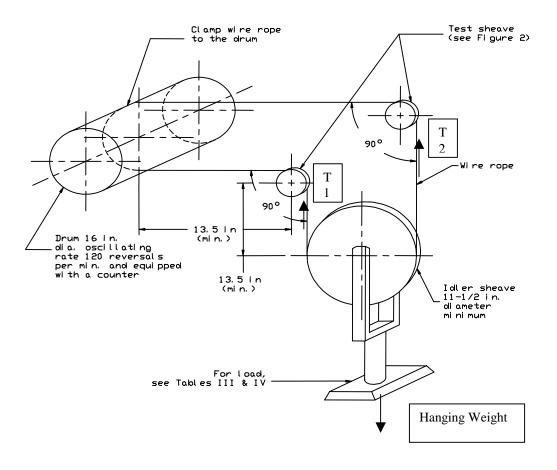
NOTE: The dimensions of the test sheaves are test parameters only and are by no means intended as design criteria. For test loads, see tables III and IV.
