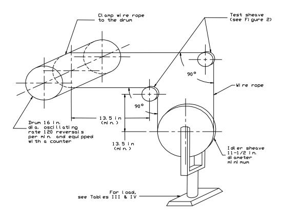
NOTE: The dimensions of the test sheaves are test parameters only and are by no means intended as design criteria.
