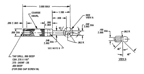
FIGURE 1. Plug, for types I and II grounding assemblies.
