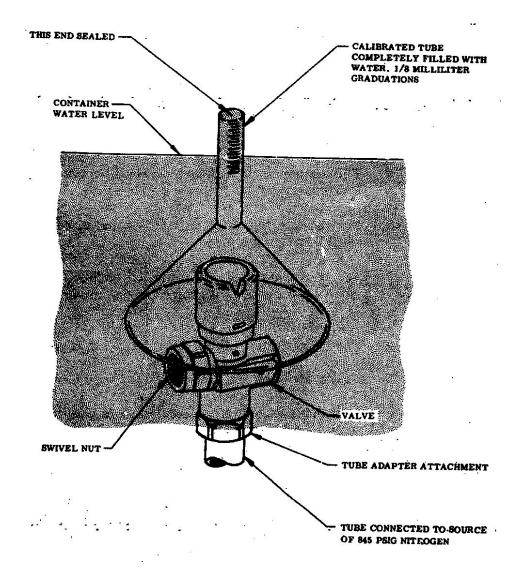
FIGURE 5. Apparatus for determining leakage at 70 °F.
