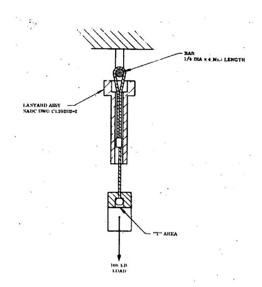
FIGURE 6. Lanyard pull test.
