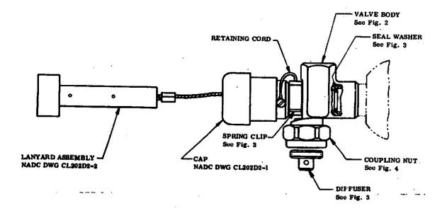
FIGURE 1. <u>Inflation valve assembly</u>.
