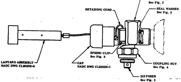
FIGURE 1. Inflation valve assembly.
