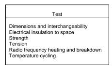
4.3.2.2.1 <u>Sampling plan</u>. Statistical sampling and inspection shall be performed on an inspection lot basis with a random sample of waveguides selected in accordance with table III. The acceptance levels shall be based upon the zero defective sampling plan. No failure shall be permitted.
