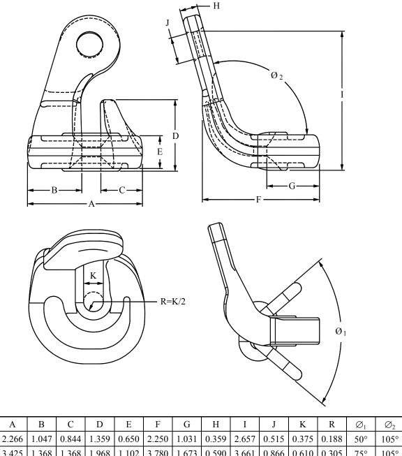
II 3.425 1.368 1.368 1.968 1.102 3.780 1.673 0.590 3.661 0.866 0.610 0.305 75° 105° Tolerances: A maximum; B, C, D, E, F, G and I approximate; H + 0.04/- 0 inch; J and K + 0.028/- 0.028;  $\emptyset_1$  and  $\emptyset_2$
