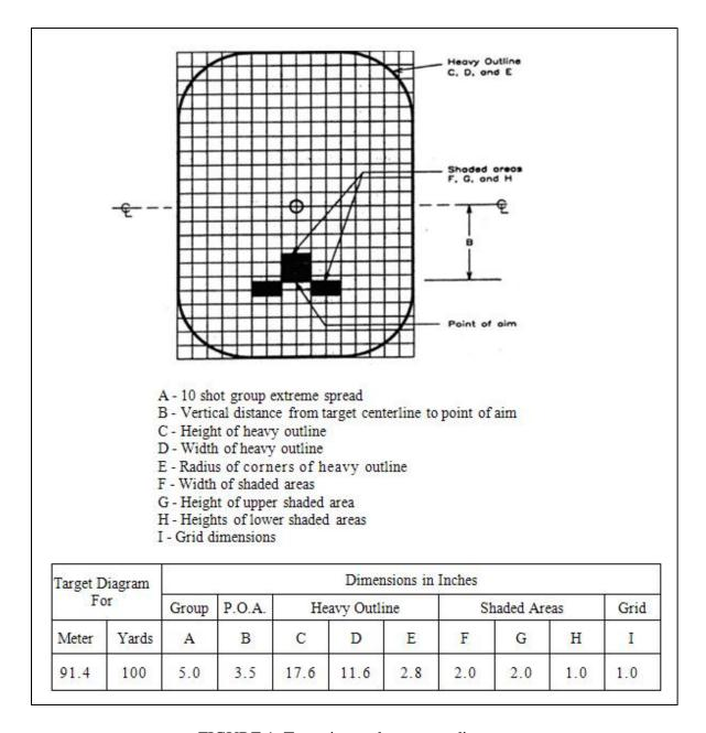
FIGURE 1. Targeting and accuracy diagram
