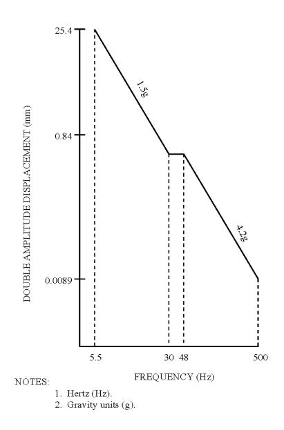
FIGURE 1. Vibration test curve.
