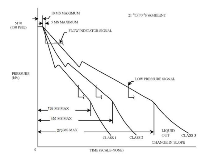
FIGURE 3. Pressure recession curves.
