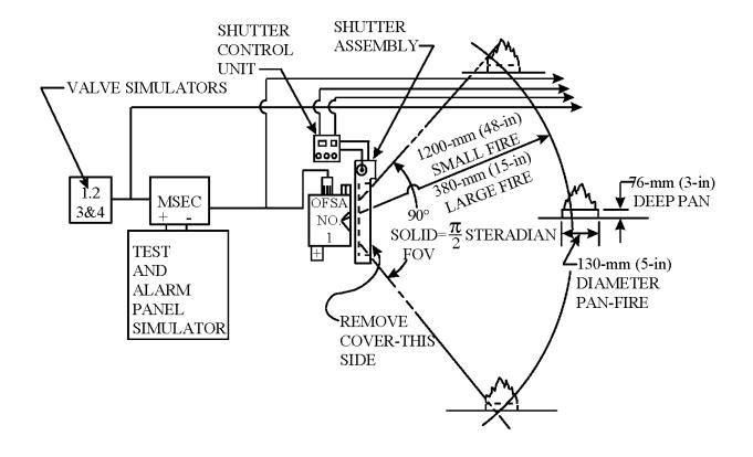
NOTE: Use of shutter assembly and shutter control unit is optional.
