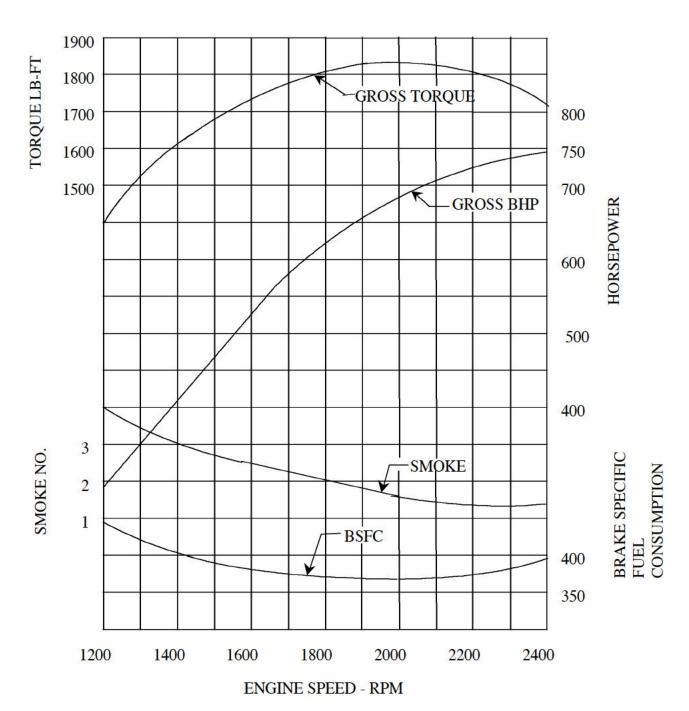
(Corrected to 29.92 in. Hg (abs.) Pressure and 60° F Temperature Ambient)
